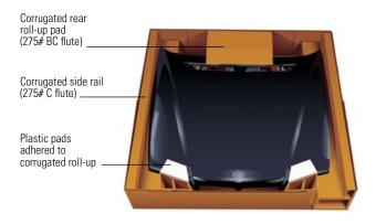
This design incorporates side rails to elevate and suspend the hood. The air space created by the elevation helps protect the grill from external forces.
