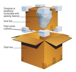
You may choose to use foam corner cushioning specifically designed to properly cushion your product during shipping. This packing method allows you to use one size of inner box, one size of outer box, and one type of foam corner cushioning to ship items of various sizes and weights.
